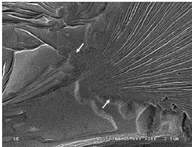
Figure 2. Relatively low magnification SEM image showing fan-shaped growth of \alpha -lamellae from the \beta growth front.
